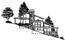
Figure 5. Terrain adapted architecture responds to the natural slope of the hillside, minimizes grading, and reduces the visual impact of the building.
